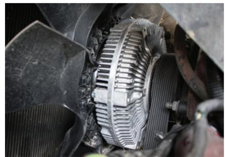
The Horton RCV250 installed on a TDS truck engine
